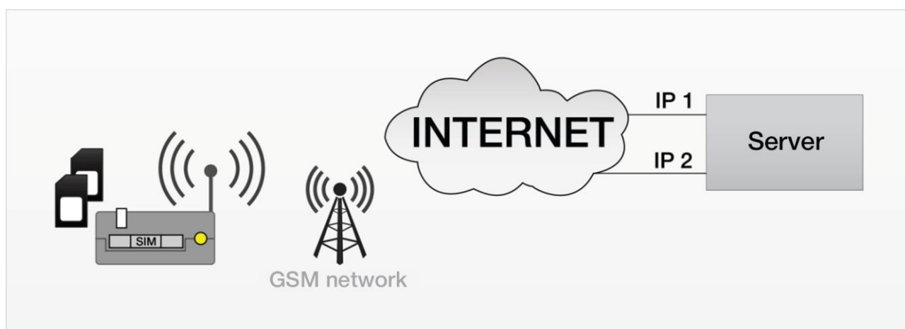
Fig. 4.4 The Diagram of Operation with Two IP Addresses on One Server
